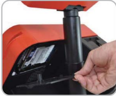
Easily Removable HDD (1 Screw)
