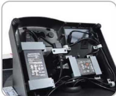
Separated Power Adaptors & Neat Cable Routing
